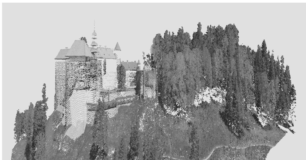
Fig. 1. The LiDAR point cloud of medieval castle near Rakow, Poland
